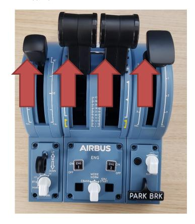
8. Make sure the 2 throttles are on TO/GA position THEN press **EACH** red buttons to set buttons 9 & 13
