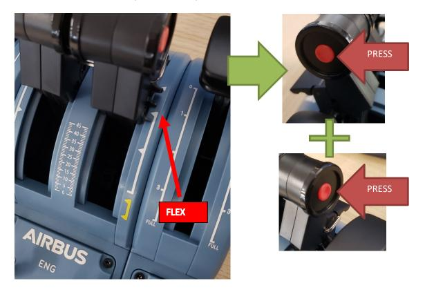
10. Move the throttles to CLB position THEN press both red buttons to set buttons 11 & 15
