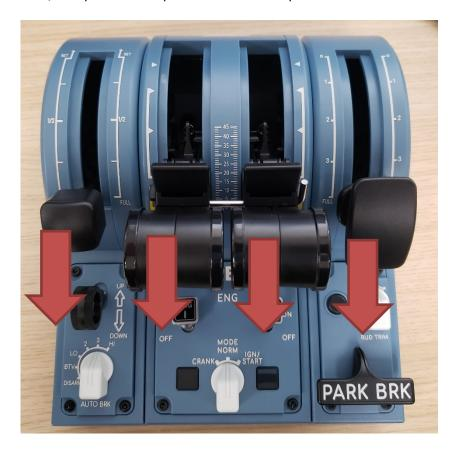
6. By having the firefault2 button pressed down, plug the device to USB to enter in calibration mode
