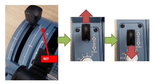
13. Move the spoiler arm to 3/4 position, activate Landing Gear, then deactivate it (UP then DOWN) to set button 28
